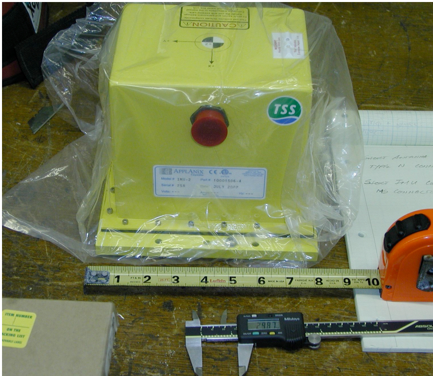
Figure 3: The POS/MV Inertial Measurement Unit (IMU.) The scale on the tape is inches.
