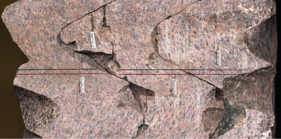
Digital scan of unrolled core of ultrahigh pressure metamorphic rocks from the Chinese Continental Scientific Drilling Project mainhole, Donghai, China (Photo courtesy of ICDP)
