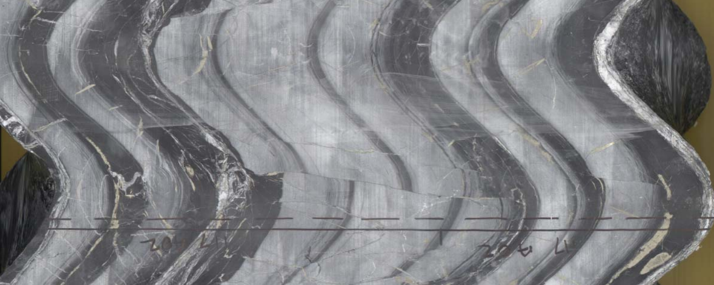
Digital scan of an unrolled core of silicious metapelite with graphitic-rich bands, Long Valley Exploratory Well Phase III, California, U.S.A. 7615' deep (Photo courtesy of ICDP)
