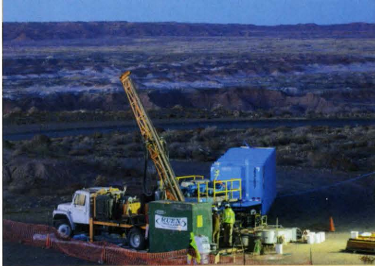
The research team's coring drill, seen here at sunset, bores deep into Arizona's Painted Desert to extract ancient stone. By the end of the monthlong project, workers had drilled through 1,700 feet of rock.
