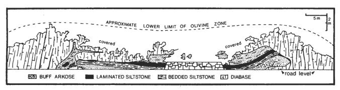
Fig. 39 Exposures of discordant contact of Palisade Diabase and Lockatong Formation, south of George Washington
