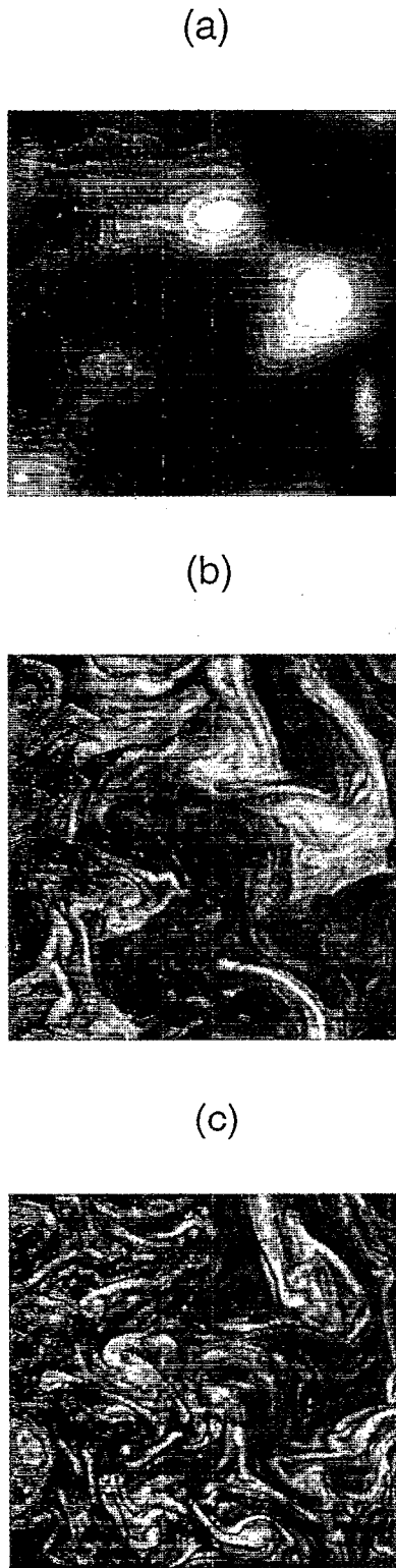
FIG. 4. Contour plots of the (a) potential \tilde{\phi}(x,y) , (b) density \tilde{n}(x,y) , and (c) vorticity fluctuations \tilde{\Omega}(x,y) at the same instant of time in a saturated turbulent state for \mathcal{E}=0.1 , \nu=10^{-8} , K_0=0.15 , and 512^2 grid points. The figures show only the region [0:\pi L] \times [0:\pi L] .
