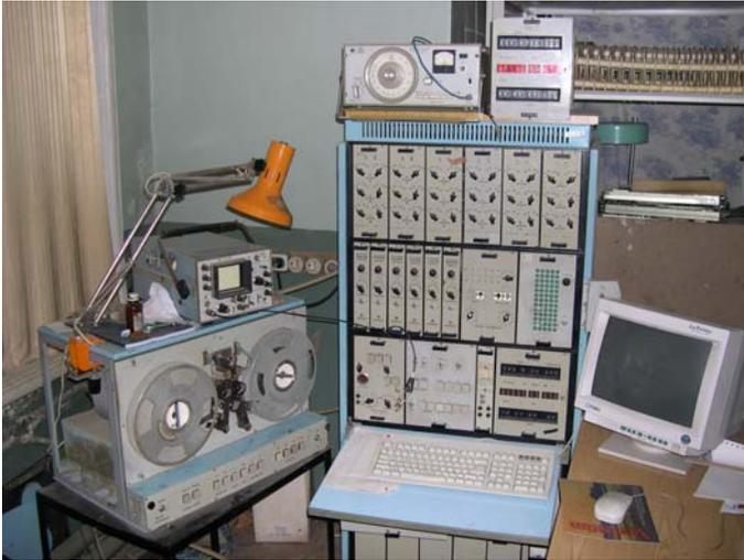
Figure 2. Playback and digitizing system for CHERPAKHA seismographs (GEON Center, Moscow, 2004).
