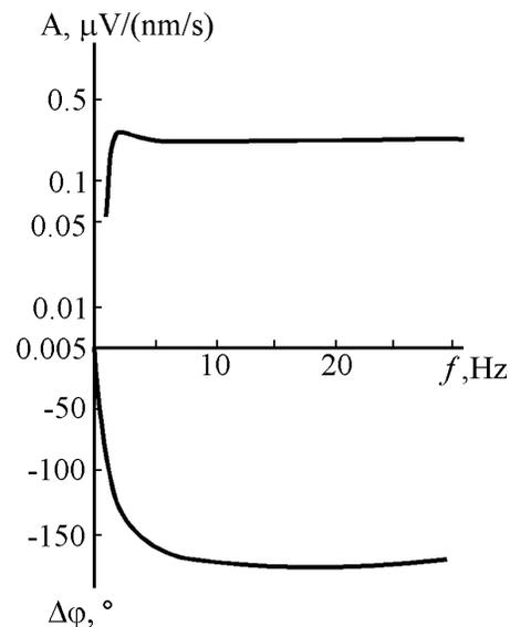
Figure 3. Amplitude and phase responses of “Taiga” recorders with NSP-1 seismometers used in DSS PNE recordings (after Ryaboy, 1989).
