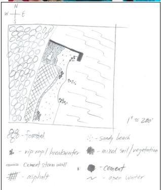
**Location:** Bloomers Beach – north end **Area:** sandy beach, banks altered, pier with rip rap sections, wood bulkhead, collected wood/debris in area, piping approx. 30" located at sampling site, 2 stone breakwaters as well as on shoreline, + cement storm wall
