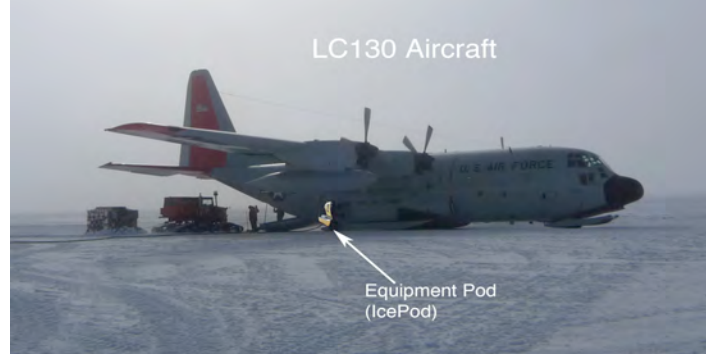
Image 5) The Ice Pod project LC130 Aircraft outfitted with radar mounted on an external 'pod' to collect images of the ice layers and the bedrock surface below. (edited image by R. Bell)
