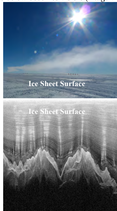
Image (7 top) The East Antarctic ice sheet and a radar image (bottom). Radar allows us to see below the ice surface, through the internal ice layers to these mountains ~2000 m below!
