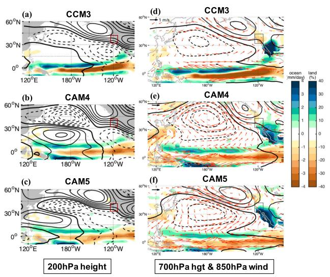
FIG. 8. OBS minus FRCST differences of FMA 2016 ensemble mean precipitation (shaded; mm day<sup>-1</sup> over ocean and percent of climatology over land) with (a)–(c) 200-hPa geopotential height (contour; 5-m interval) and (d)–(f) 700-hPa geopotential height (contour; 5-m interval) and 850-hPa wind (vectors).
