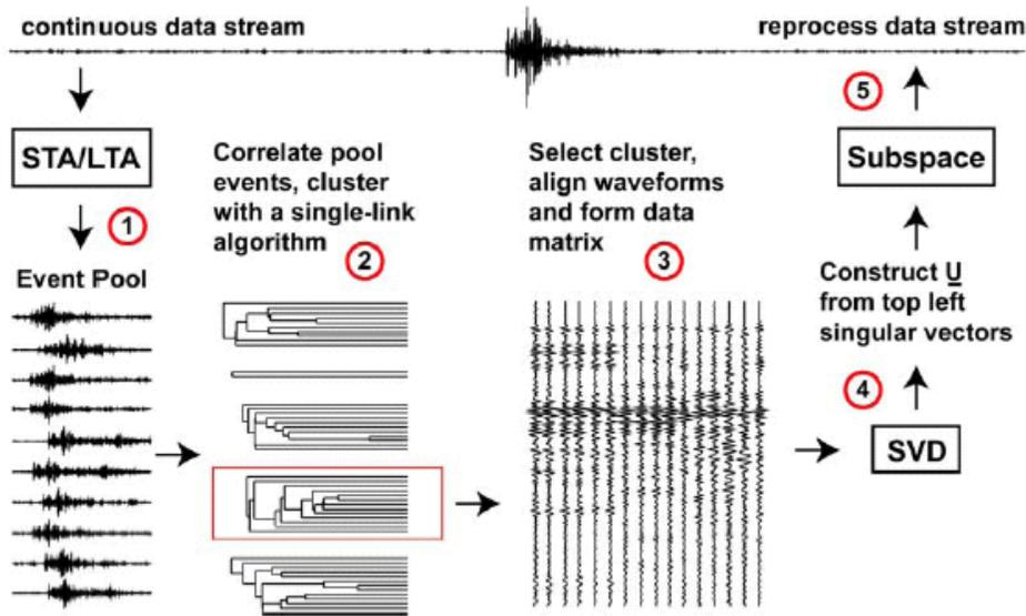
Figure 5. A “bootstrap” procedure for designing and applying subspace detectors empirically to reduce the detection threshold for a specific source with five steps.
