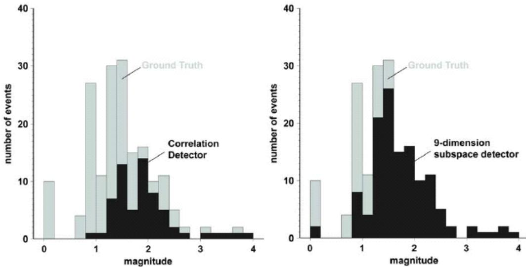
Figure 7. A 9-dimension subspace detector detected twice as many San Ramon swarm events as the correlation detector when both were operated at the same theoretical false alarm rate. The histograms above compare the distribution of detections by magnitude to the ground truth event distribution obtained from the BSL catalog. The subspace detector has a threshold around Md 1.5 at 240 kilometers range.
