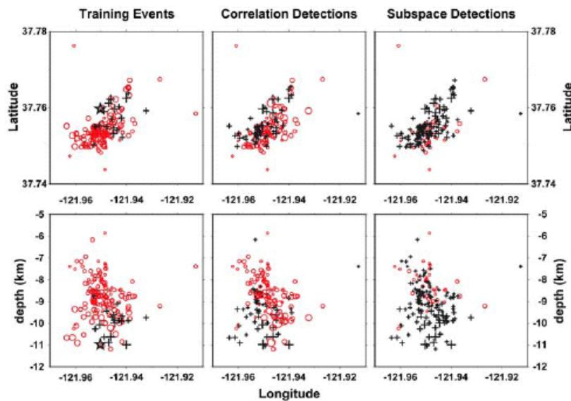
Figure 8. Subspace algorithm detections have broader spatial distribution than the correlator detections, but both miss a large fraction of the shallower events in the sequence. The maps above show the distribution of San Ramon sequence events in latitude and longitude (top maps) and in longitude and depth (bottom maps). The maps at left show the distribution of master events used in the design of the correlator (star) and subspace detectors (star and crosses).
