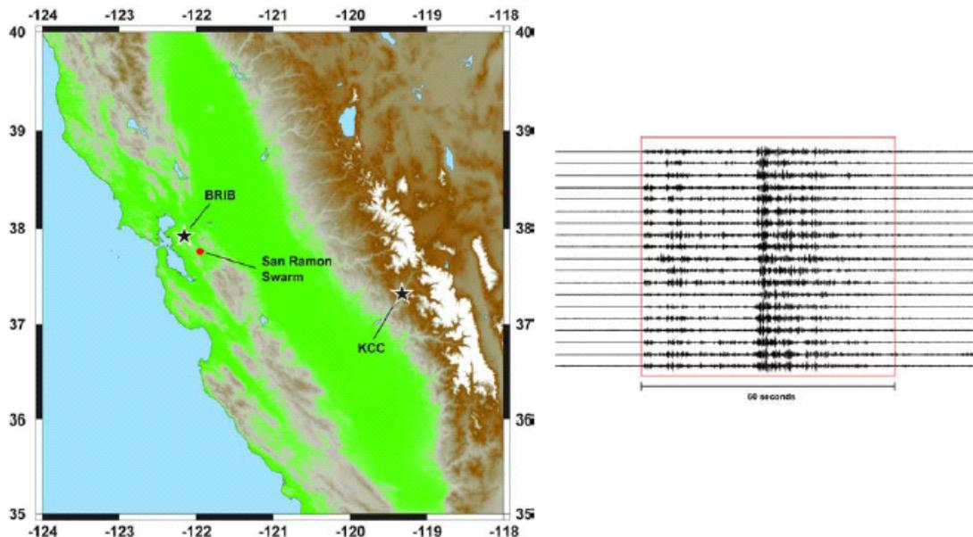
Figure 6. The 2002 San Ramon, California, swarm provided a convenient test of subspace detector design and performance. Data from two Berkeley Digital Seismic Network broadband stations (KCC, BRIB) were used in the test example to implement the detector and help assess its performance. At right are the waveforms of the 19 events used to develop subspace detectors and a correlator. A degree of signal variation is evident in the waveforms.
