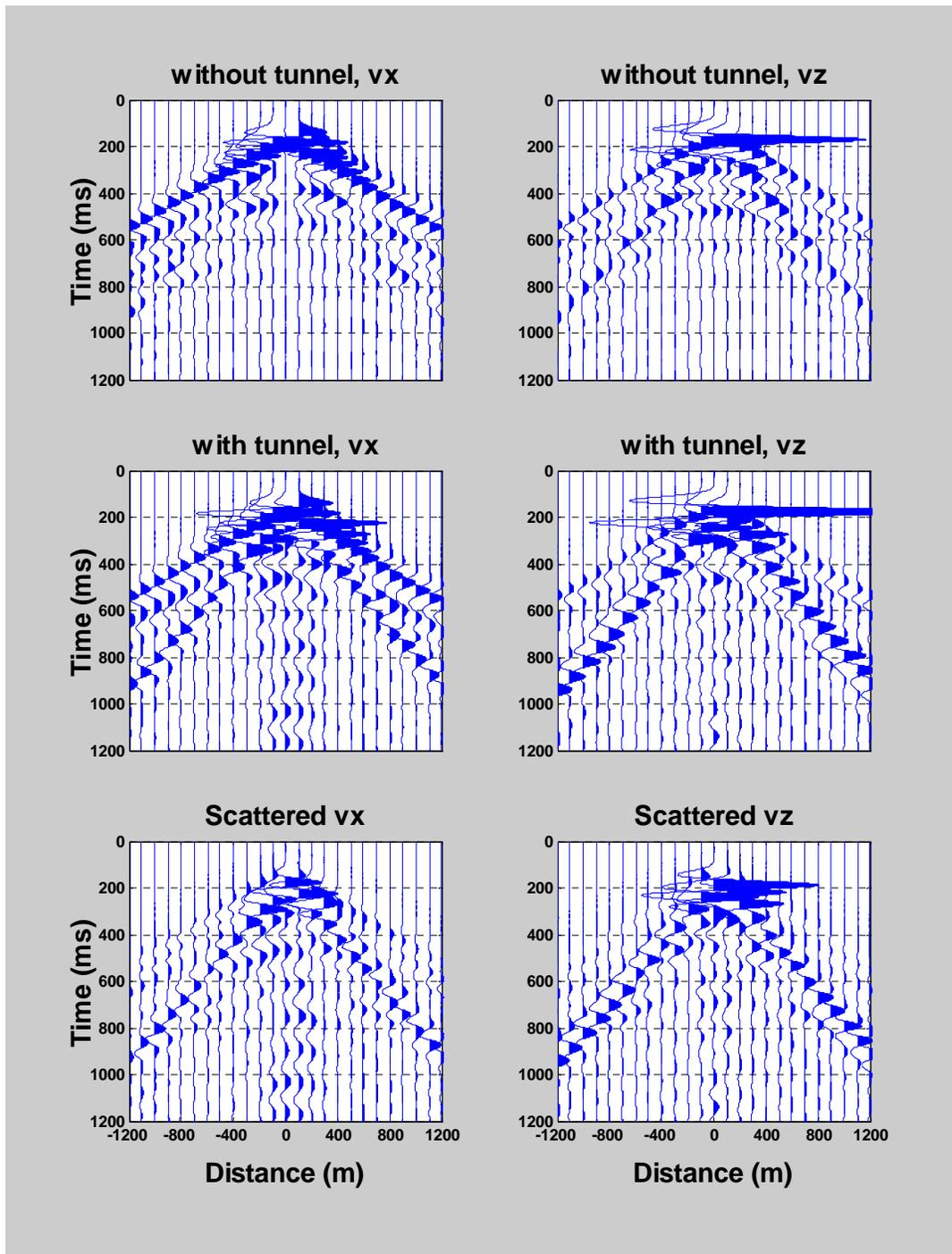
Figure 2. Comparison of the x and z components of the velocity fields at the free surface in the absence and the presence of the tunnel. Respective scattered velocity fields of the x and z components, obtained by subtracting row 1 from row 2, are also shown in the last row of this figure.
