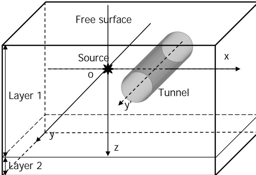
**Figure 1.** The geometry diagram of the tunnel model. The explosion source is located at 100 meter deep. A cylindrical tunnel is set 30 m away from the source, with radius of 15 m and length of 50 m. Its symmetric axis is parallel to the y axis. The receivers are set on the free surface. The distance between the adjacent receivers in x or y axis direction is 100 m.
