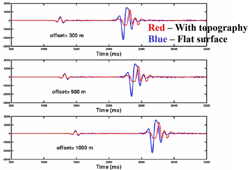
**Figure 4b. Comparison of waveforms for an explosion/tunnel under a flat free surface and under a hill.**
