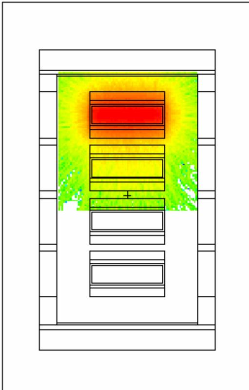
Figure 1. Map of photon flux from  $^{133}\text{Xe}$  source in top chamber of  $\beta$ - $\gamma$  coincidence detector MCNPX model.
