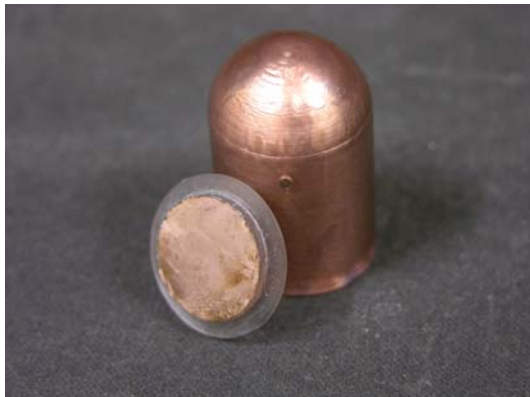
Figure 1. Photograph of copper-coated plastic scintillating gas cell and endcap for detection of \beta radiation. Only the interiors of the cell and endcap are metallized.
