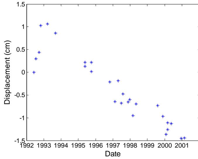
**Figure 4. Cumulative displacement along radar line-of-sight since May 5, 1992 for London tunneling area identified by arrow in previous figure. Positive (negative) displacement represents movement toward (away from) radar.**
