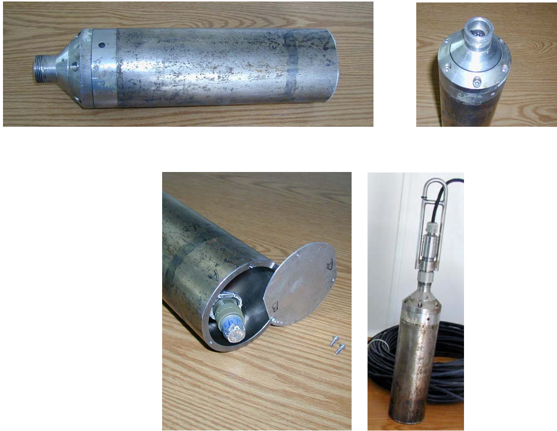
Figure 2. Sensor Impedance Simulator with interchangeable loads.
