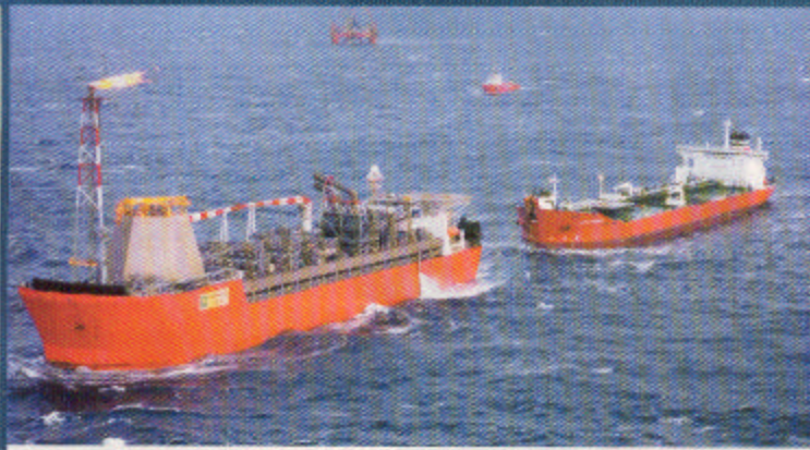
TANDEM OPERATION: THE SCHIEHALLION TRAILED BY A SHUTTLE TANKER, WHICH DELIVERS OIL TO THE MAINLAND.
