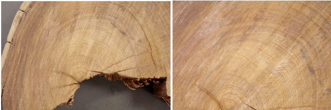
Figure 2. Two views of a section of Pterocarpus erinaceus from Senegal collected in March 2007 by D. Blanas showing visible ring structure.
