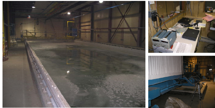
Figure 1. Images of the CRREL test basin from September, 2007. The 37 m sea ice tank is pictured on the left. Guides on both sides of the basin allow for the lateral placement of the instrument gondola whose exterior and interior are pictured on the lower and upper right, respectively.
