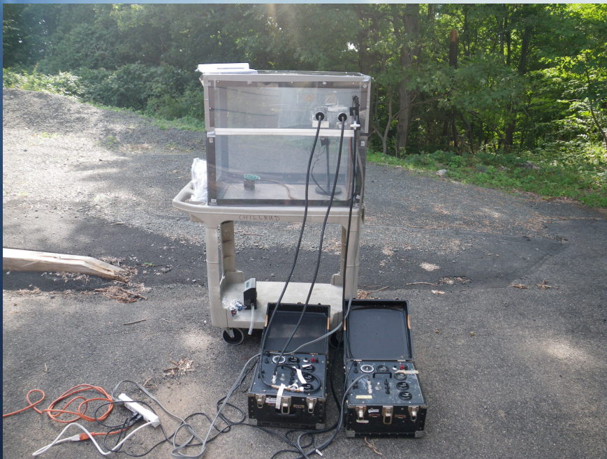
Figure 1: Combustion chamber where incense smoke samples collected
