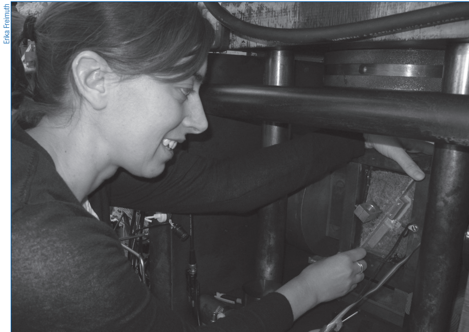
In the recently renovated rock mechanics lab, Heather Savage slides two wedges of rock into a biaxial deformation apparatus, which applies pressure until the two pieces slip. Attached wires record displacement and acoustic emissions, allowing Savage to model the behavior of faults under stress.
