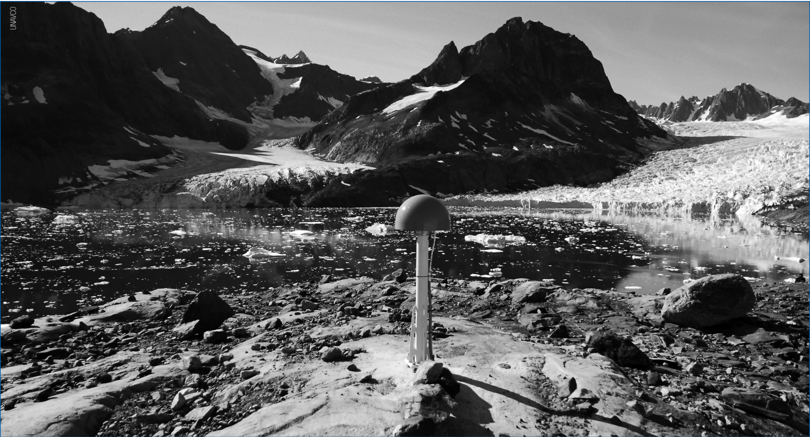
A GPS antenna sits atop a single mast bolted to the bedrock in eastern Greenland.
