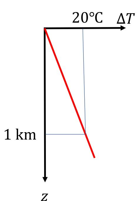
(A) surface heat flow of q=0.06 W/m<sup>2</sup> implies hotter temperatures at depth, increasing by about 20 degC / km
