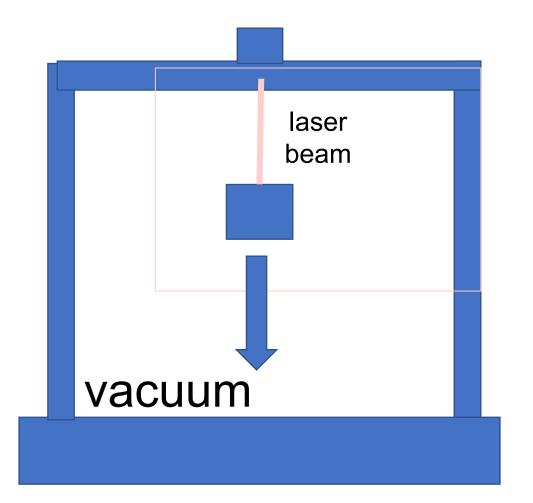
measure acceleration optically with laser interferometry
