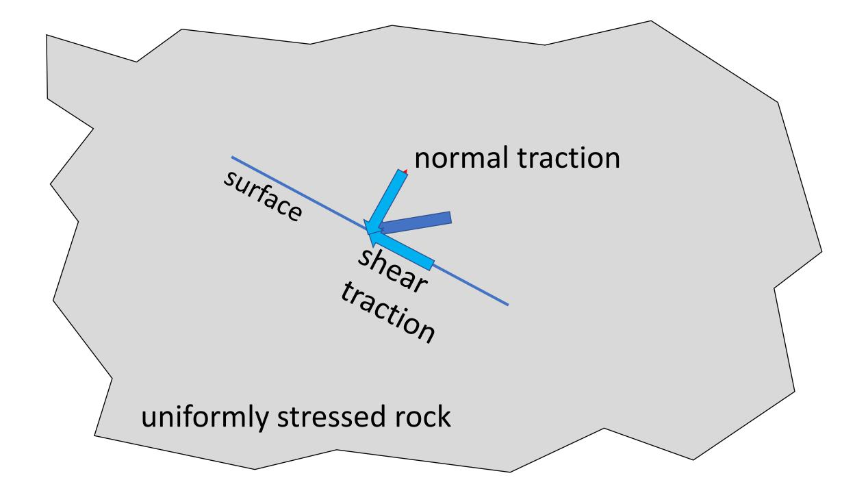
It is always possible to identify three surfaces with no shear tractions
