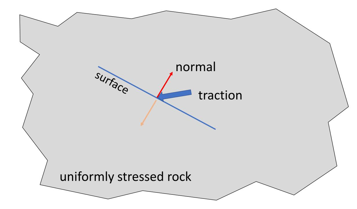
Tractions on two sides of a surface are equal and opposite
