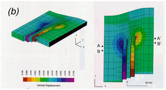
Figure 3. An example, taken from ten Brink et al. (1996) of the use of the Beasy code in a geophysical context. Here the displacements around strike slip faults that intersect the surface of the earth are modeled. (A) The horizontal displacement of the earth due to a strile slip fault. (B) The vertical displacement due to several interacting facults. The grid represents deformation of the originally orthogonal mesh.
