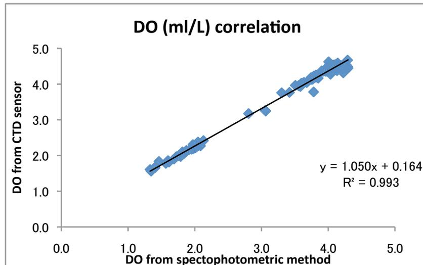
Figure 2. Comparison of DO obtained using the Spectrophotometric method and the CTD DO sensor
