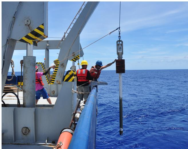
Figure 12. The OSU gravity corer during retrieval.
