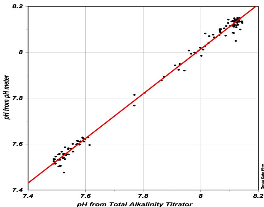
Figure 3. Comparison of pH obtained using the pH meter and total alkalinity titrator
