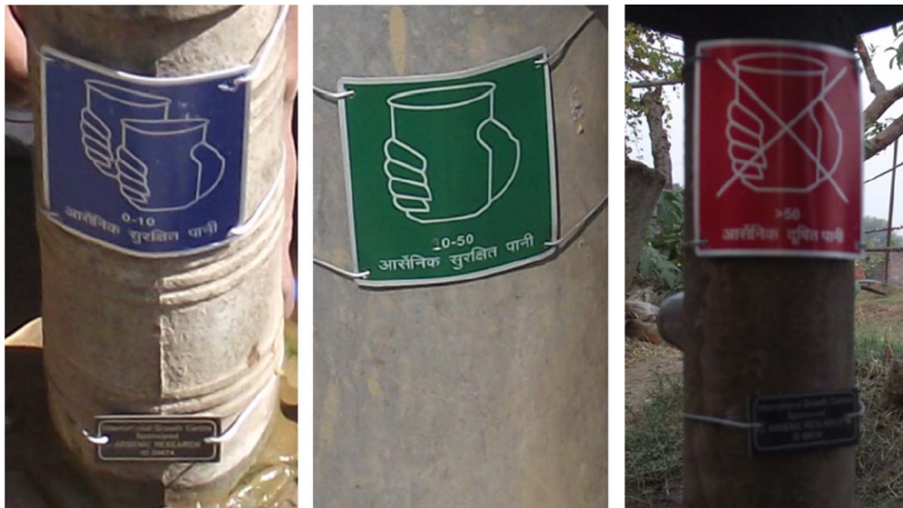
Figure 3: Metal Placard showing arsenic status after testing
