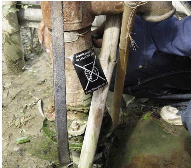
Fig. 1. Tube well and test result plate. The picture shows an example of the black-and-white plate used to communicate results: the plate indicates the well I.D., the year when the water sample was taken, the arsenic level and a hand holding a drinking cup, in this example crossed out because the arsenic level (336 ppb) is above the safety threshold. The smaller, stainless steel plate visible above the black-and-white one indicates the well I.D. and was attached to the well in 2005, at the time of the water sample collection.
