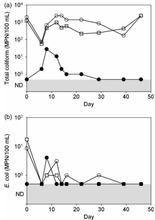
**Figure 4** | Timeseries of (a) total coliforms and (b) *E. coli* concentrations within the pumped water discharge of the previously used hand-pump (no. 21602). Sterile artificial groundwater (50 L) was flushed daily through the hand-pump. Water samples were collected from the 1st (○) and 20th (□) strokes and directly from the reservoir after pumping (●). The reservoir was cleaned and refilled with sterile AGW after each sampling event.
