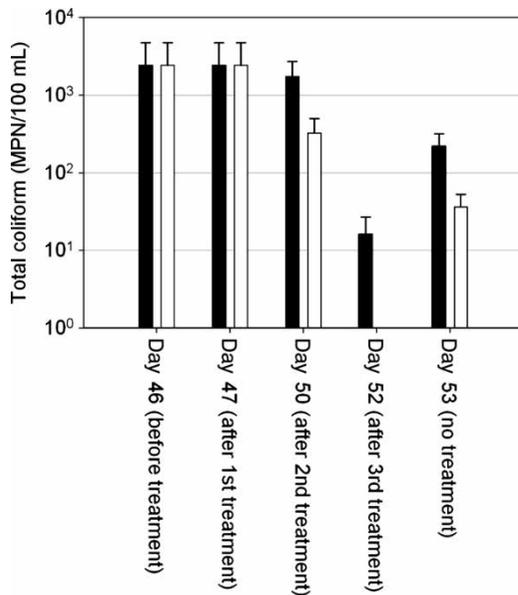
**Figure 6** | Concentration of total coliforms in discharge from hand-pump no. 21602 on day 46 (before treatment), day 47 (after the first round of shock chlorination), day 50 (after the second round of shock chlorination), day 52 (after the third round of shock chlorination, combined with acid soaking and aggressive scrubbing) and day 53 (no treatment). Enumeration of total coliforms was determined following the 1st (■) and 20th (□) strokes. Error bars represent 95% confidence intervals.
