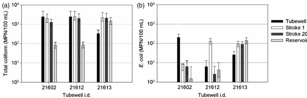
**Figure 3** | Concentration of (a) total coliforms and (b) *E. coli* in discharge from the previously used hand-pumps prior to removal from their corresponding village tubewell, and following their attachment to reservoirs containing 50 L of filter-sterilized groundwater. Discharge from the reservoir-attached samples was collected on the 1st and 20th hand-pump stroke. Samples were also collected directly from the reservoirs after pumping. Error bars represent 95% confidence intervals.
