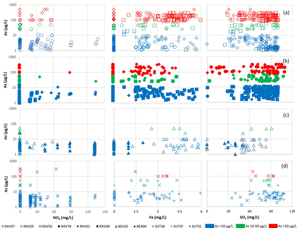
Fig. 4. Relation of As with other field parameters in Indus basin, Punjab, India. Villages are in the same order and use the same symbols and color code as in Figs. 3a–3d: (a) RAV06, RAV50, RAV92 in northern Ravi; (b) RAV82, RAV63, RAV09 in southern Ravi; (c) BEA06, BEA00 in Beas; (d) SUT05, SUT28, SUT01 in Sutlej. The samples up to 50 m depth are only shown.
