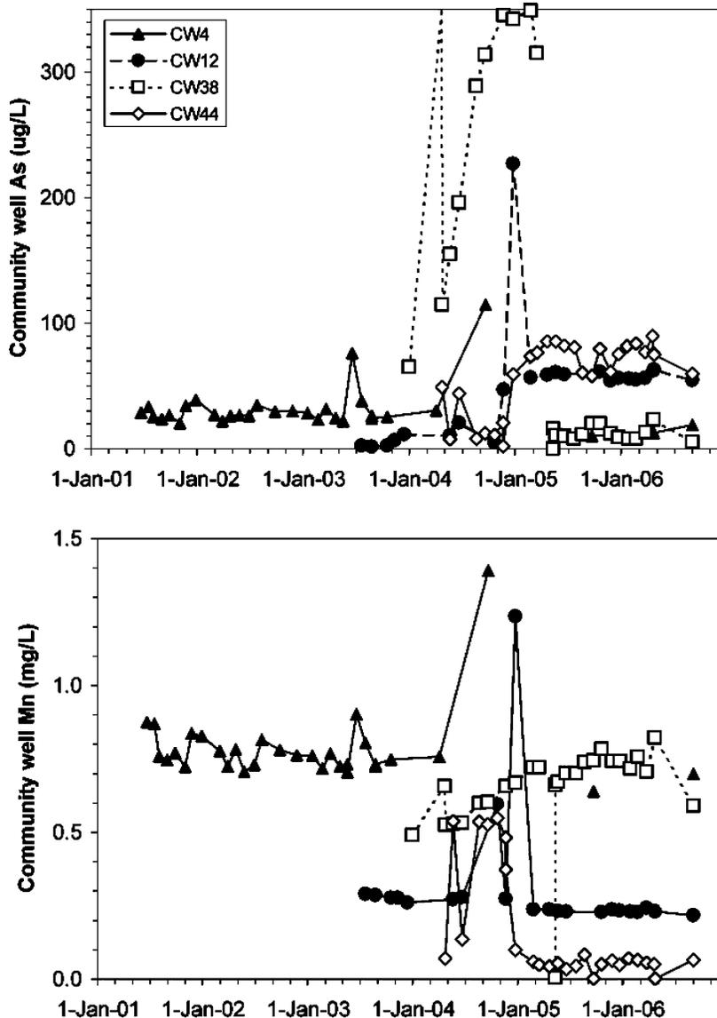
**Fig. 5.** Monthly variations in As and Mn content of groundwater pumped for wells CW04, CW12, CW38, and CW44. Wells CW04 and CW38 were re-installed to the same depth in June 2004 and March 2005, respectively.
