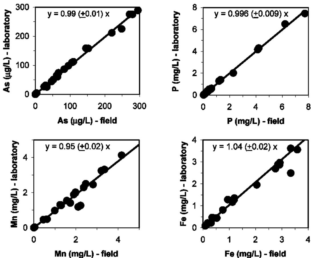
Fig. 3. Comparison of groundwater analyses for duplicate samples from tubewells of Araihasar, one of which was acidified immediately and the other 11 months later in the laboratory (Table 1).
