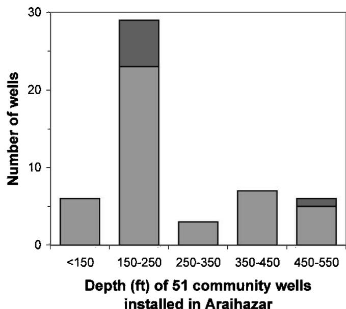
**Fig. 2.** Histogram of the depths of 51 community wells installed in Araihasar, distinguishing wells installed in sandy deposits that are orange-brown (light shading above) from wells installed in white or grey sands (dark shading).
