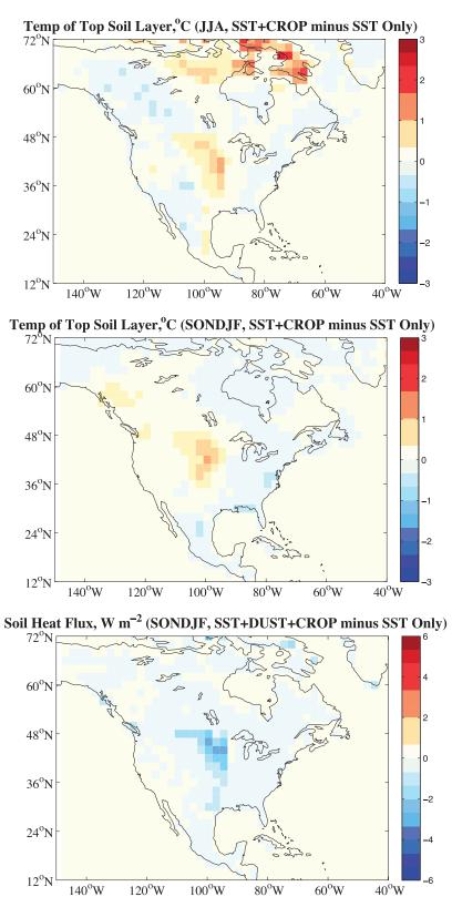
**Fig. S4.** Difference (SST+CROP – SST-Only) in temperature of the top soil layer for June–August (JJA, *Top*), September–February (SONDJF, *Middle*), and difference in soil heat flux for September–February (SONDJF, *Bottom*). Negative soil heat flux values indicates an anomalous heat flux directed from the soil to the atmosphere.
