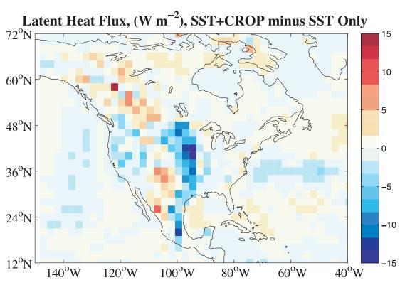
Fig. S3. Difference in sensible (*Upper*) and latent heating (*Lower*) for the June–July–August period (SST+CROP minus SST-Only). Reductions in vegetated area from crop removal reduce transpiration and total surface water fluxes, shifting the surface energy balance to favor sensible over latent heating.
