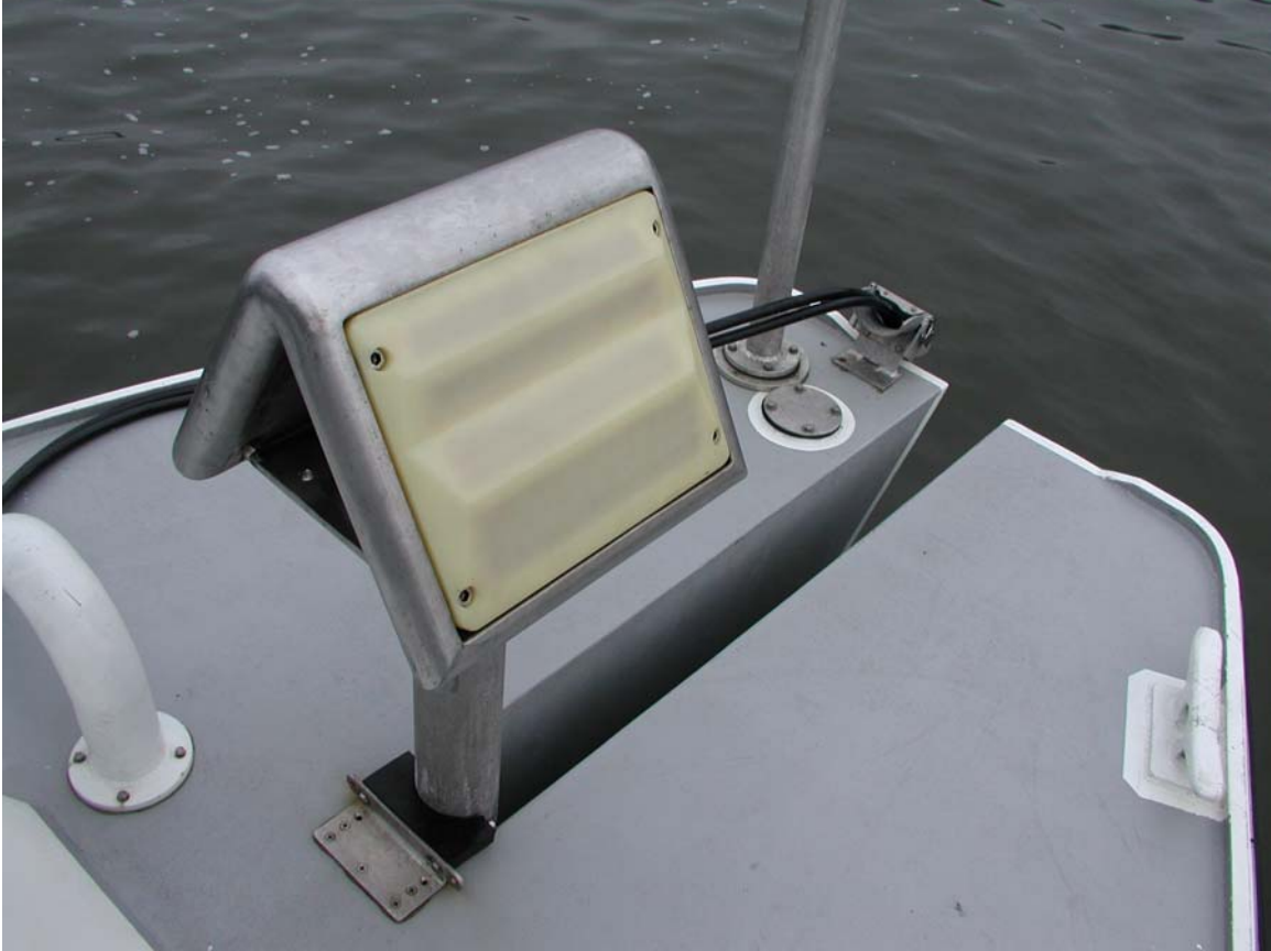
Figure 3: The Fansweep20 transducer in the stowed position in the custom-made bow. A hydraulic mechanism tilts the transducer 180 degrees through the slot into the working position.
