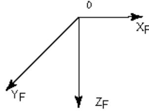
and consider a body reference frame with X positive toward the bow, Y positive to starboard, and Z positive pointing toward the center of the earth:
