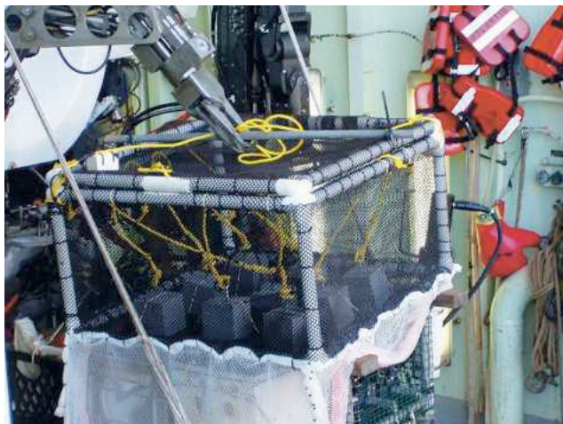
Figure 2. The mussel exclusion cage on the basket of Alvin before deployment on the bottom at the Marker 119 study site. The nine basalt settlement blocks are kept in place with rubber bands and have a nylon rope attached to an embedded eyebolt for later retrieval with the manipulator arm of Alvin . The weighted, netted skirt around the bottom of the exclusion cage serves to seal the cage to the uneven seafloor, inhibiting the migration of mussels under the cage.
