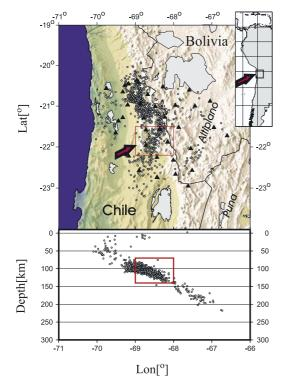
**Figure 1.** Map of the Central Andes, showing passive seismic stations of the 1996 ANCORP experiment (black triangles). 1050 locally recorded seismic events (open circles) were manually inspected and located. Lower panel shows a depth section of the seismicity located using a 3-D velocity model [*Rietbrock and Haberland*, 2001]. Red squares include the events analysed in this study.
