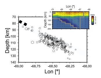
**Figure 2.** 240 earthquakes located by a 3-D tomographic inversion of P- and S-phase arrival times. Inset shows the P-wave velocity model for the corresponding cross section. Events between  $21.5^{\circ}$ S and  $22.2^{\circ}$ S were projected onto the section (see red box in Figure 1). Size of circles corresponds to event magnitude ranging from  $M_L$  1.3 to 4.7.
