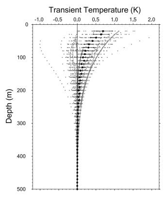
**Figure 2.** Ensemble of the transient component of subsurface temperature versus depth from each of the boreholes in the Russian data set. The mean and standard error of the mean in each 10 m depth interval is shown in bold.
