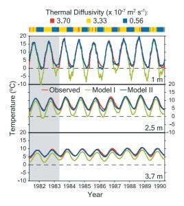
**Figure 2.** Observed and modeled temperatures at depths of 1.0, 2.5 and 3.7 m. Shaded years are tuning years, unshaded years are validation years. Time-dependent thermal diffusivity used in Model II shown in color bar at top.
