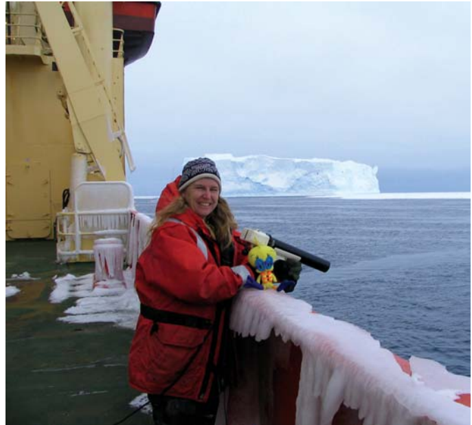
Dr. Robin Robertson collected XBT (expendable bathythermograph) and CTD (conductivity-temperature-depth) profiles on the AnSlope III field program in the Ross Sea. Here, she is aboard the RVIB Nathaniel B. Palmer launching an XBT with the mascot of the 6 th grade class at George Grant Mason Elementary School, Tuxedo, NY. She is now at Lamont-Doherty Earth Observatory of Columbia University where she further investigates vertical mixing mechanisms, particularly internal tides and waves, in the Ross, Weddell, and Indonesian Seas.
