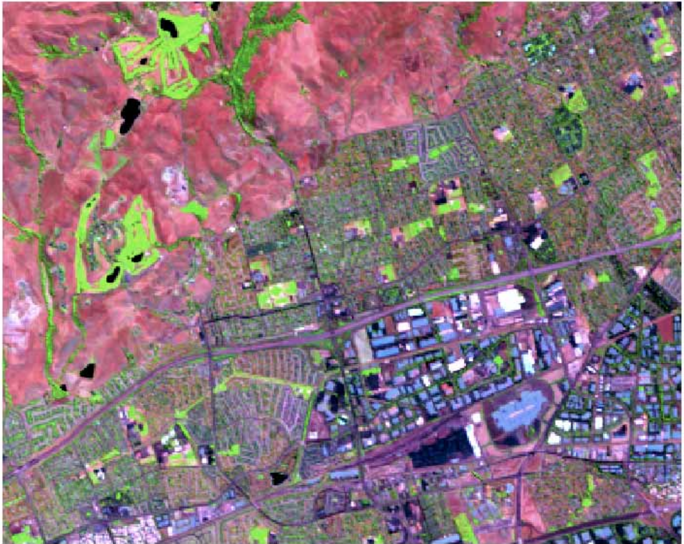
Figure 1. AVIRIS false color composite of Milpitas California acquired in 1997. The Red, Green and Blue layers correspond to the 2.21 \mu\text{m} , 0.81 \mu\text{m} and 0.66 \mu\text{m} wavelength bands respectively. The image is 6 x 8 km and each pixel is approximately 20x20 m. The spectral dimensionality of the mosaic of urban, suburban and undeveloped areas varies at scales larger and smaller than the Ground Instantaneous Field Of View (GIFOV) of the AVIRIS sensor.
