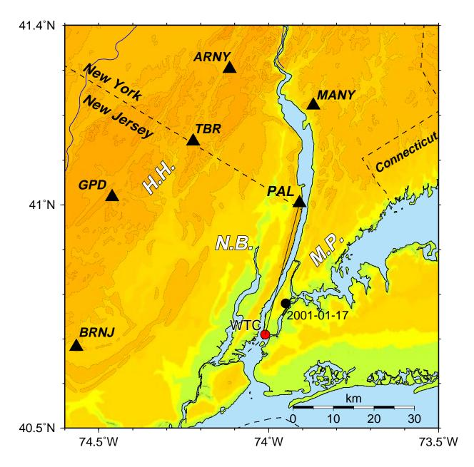
Figure 2: Seismograph stations and topography for greater New York City area. Solid triangles indicate stations that recorded events at WTC (solid red circle); black circle, epicenter of earthquake of January 17, 2001. N.B. denotes Newark basin; H.H., Hudson Highlands; M.P., Manhattan Prong.
