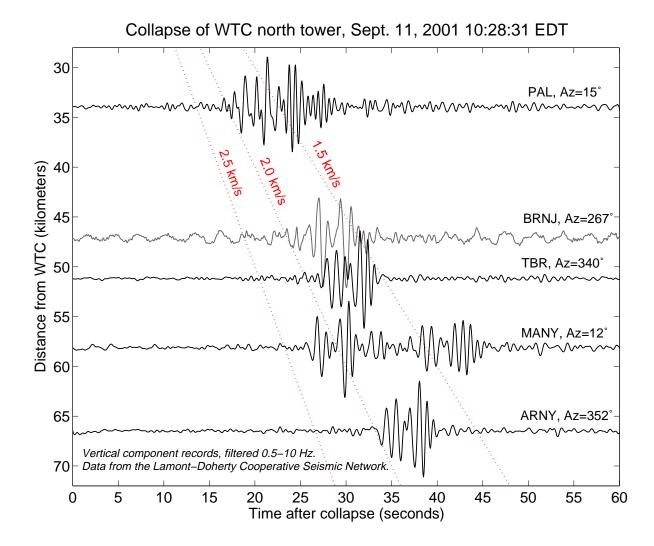
Figure 3: Record section of vertical-component seismograms from stations in Fig. 2 following collapse of north Tower of WTC. Zero corresponds to computed origin time of 10:28:31 EDT. Data filtered for passband 0.5 to 10 Hz. Three velocities indicated by dotted lines.
