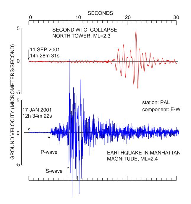
Figure 4: Comparison of Palisades seismograms for collapse 2 and earthquake of 17 January 2001. Arrows at left indicate computed origin times.
