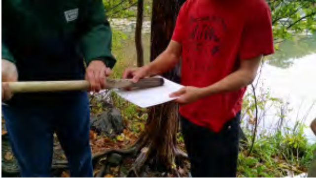
STEP TWO: Remove Sediment Core Sample from Sampling Tube
