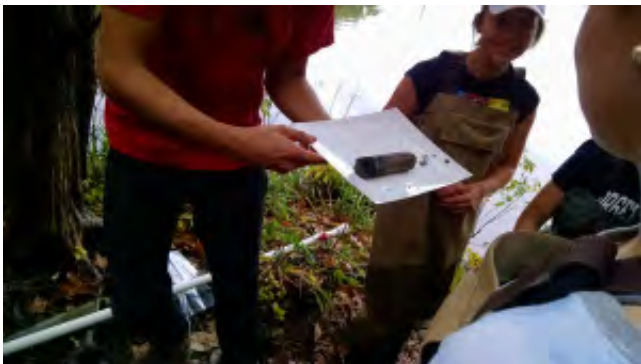
STEP THREE: Analyze the Core Sample (view, measure, smell, then send off to the lab for heavy metals analysis)
