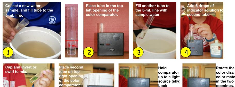
color disc until color matches in the two openings. Read pH in scale window.
