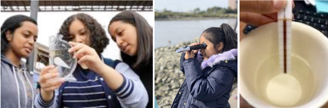
Salinity is measure using (From left to right) a hydrometer, a refractometer, or quantabs.
