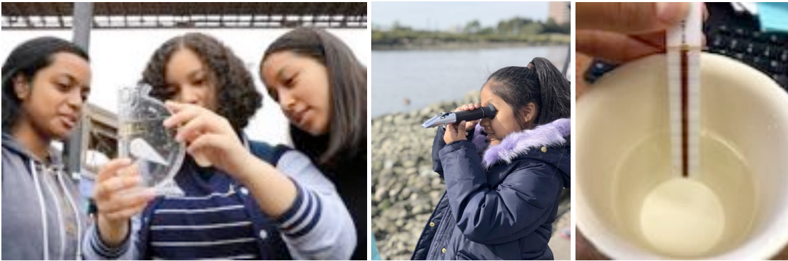
Salinity is measured using (from left to right) a hydrometer, a refractometer, or quantabs.
