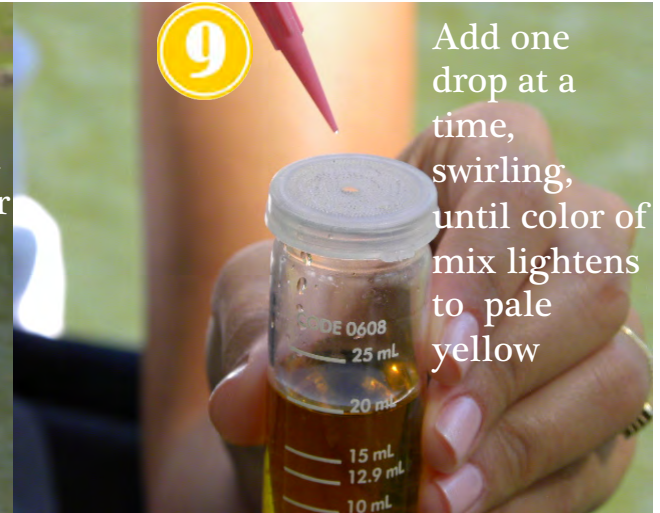
12 Continue to titrate the fixed sample using one drop at a time of the Thiosulfate from the plunger.
