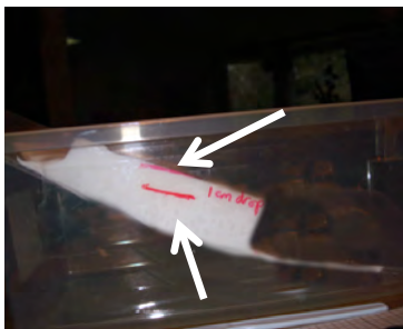
Figure 3) Place clear tape on outside of container. Mark goo surface and 1 cm below.
