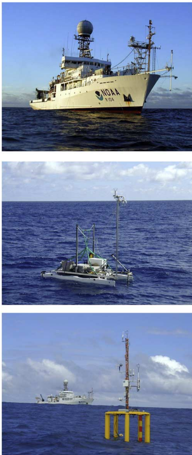
Figure 2. Floating platforms used to support flux and surface process measurements during GasEx-2001: (top) Brown , (middle) SPIP, and (bottom) ASIS.
