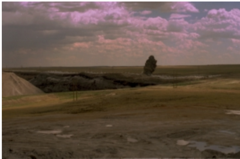
FIGURE 3. Three photos of the August 1, 1996 Black Thunder cast blast. The start at 19:33:05 (top), 1.7 seconds later (middle) and the finale at 19:33:09. The significant release of energy into the air resulted from a sympathetic detonation which occurred part way through the shot sequence.
