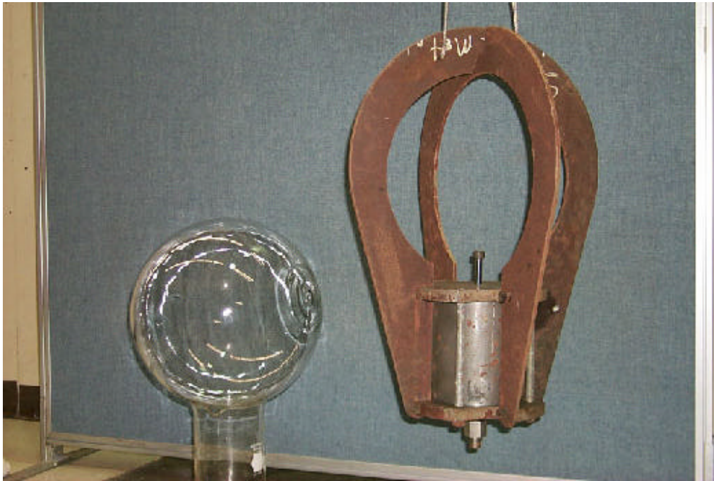
Figure 4. The spherecracker is shown on the right in the lowering orientation. The glass sphere is shown on the left atop a laboratory beaker.
