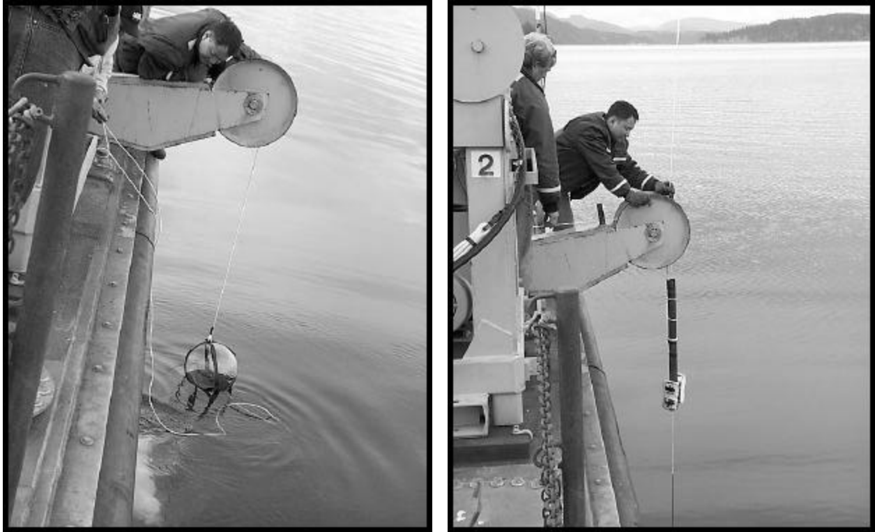
Figure 3. A 14-inch-diameter glass sphere is lowered into the water (left) during the March 1999 test conducted at Dabob Bay, WA. The sphere was lowered to a depth of 450 ft. A metal pipe was then slid down the tether line (right) in order to initiate failure. The water depth was 600-ft. Photos © by Ted Farrell.
